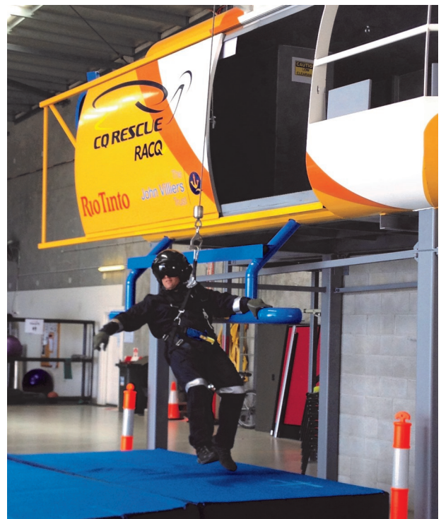
The static winch training simulator in action. Photo: RACQ CQ Rescue
